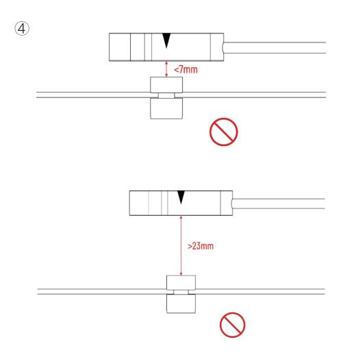
5. Adjust the speed measuring magnet to meet the above inspection requirements.
