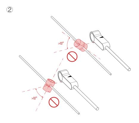
3. Check whether the speed measuring magnet is aligned with the " $\triangle$ " mark of the speed sensor.
